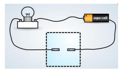
Diagram 3: Incomplete electric circuit
